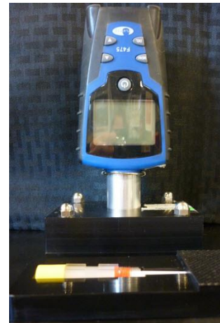
Figure 5 Grease colorimeter with cell and drawer for Full Grease Thief
