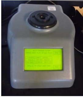
Figure 4 Grease Thief being analyzed in a ferrous debris monitor
