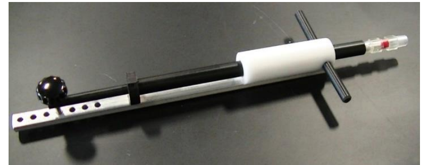
Passive Grease Sampling Device attached to a T-handle
