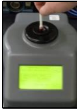
Ferrous debris level
