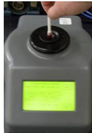
Figure 8: Hall-effect (FdM+) sensor and Grease Thief
