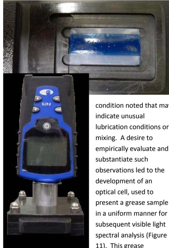
Figure 11: Spectrometer and optical cell for grease colorimetry
