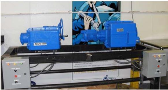
Figure 5: Motor Operated Valve (gearbox) test stand
