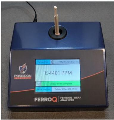
Figure 4 Grease Thief being analyzed in a FerroQ
