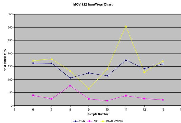
Figure 9: Steady-state wear level comparisons
