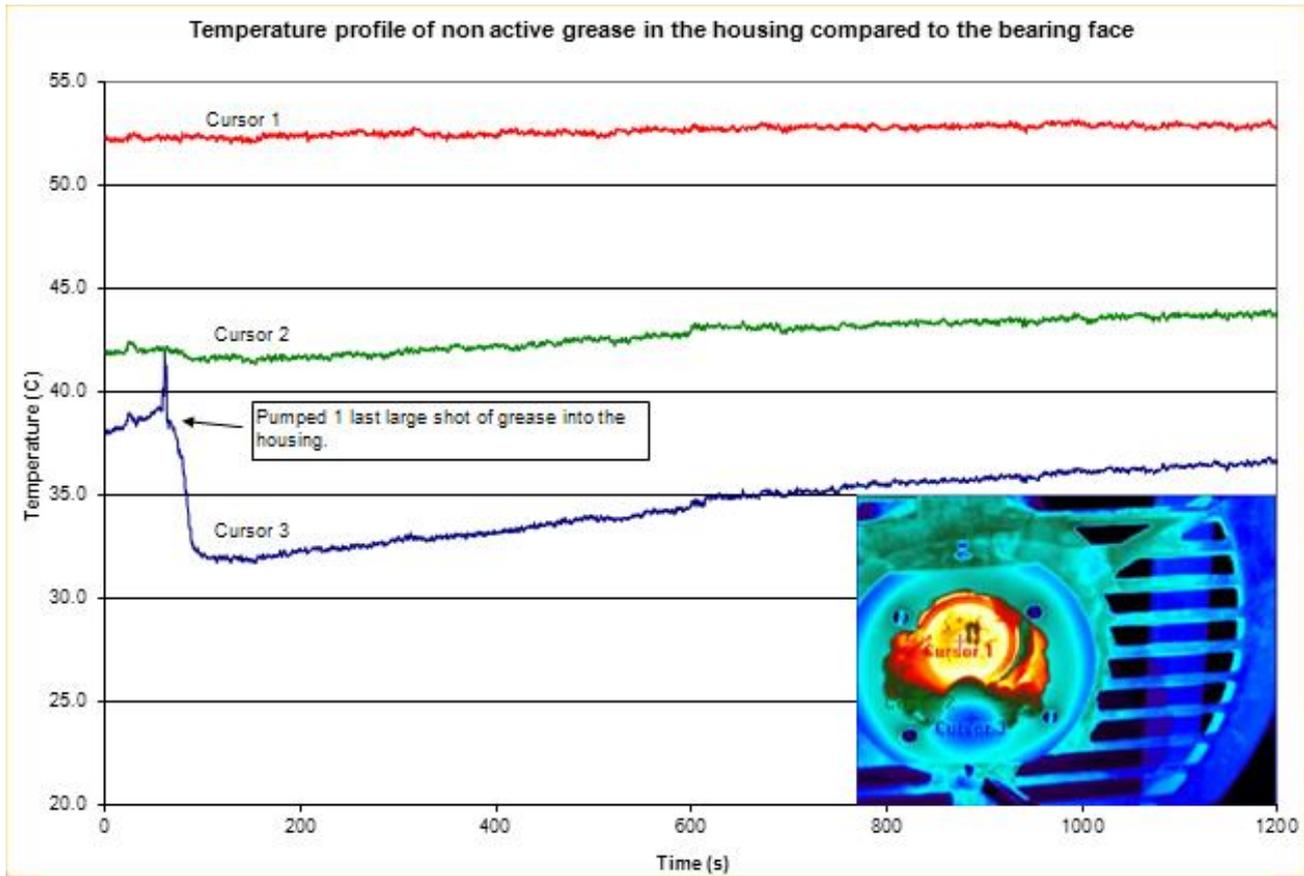
Figure 4: Profile of three selected active and non-active zones in the bearing
