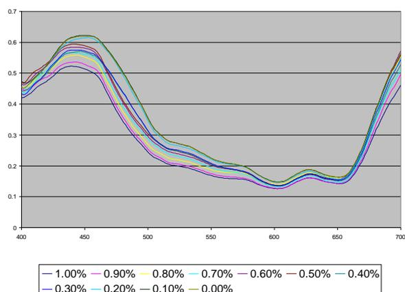
Figure 16: Spectral graphs of a grease with increasing quantity of dispersed coal dust
