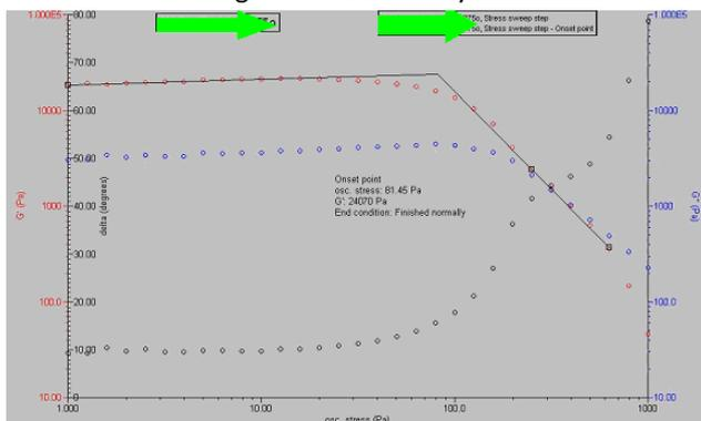
Figure 18: Oscillatory stress measurement of reference grease with cone and plate rheometer
