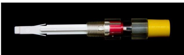
Figure 5: Passive grease sampling device
