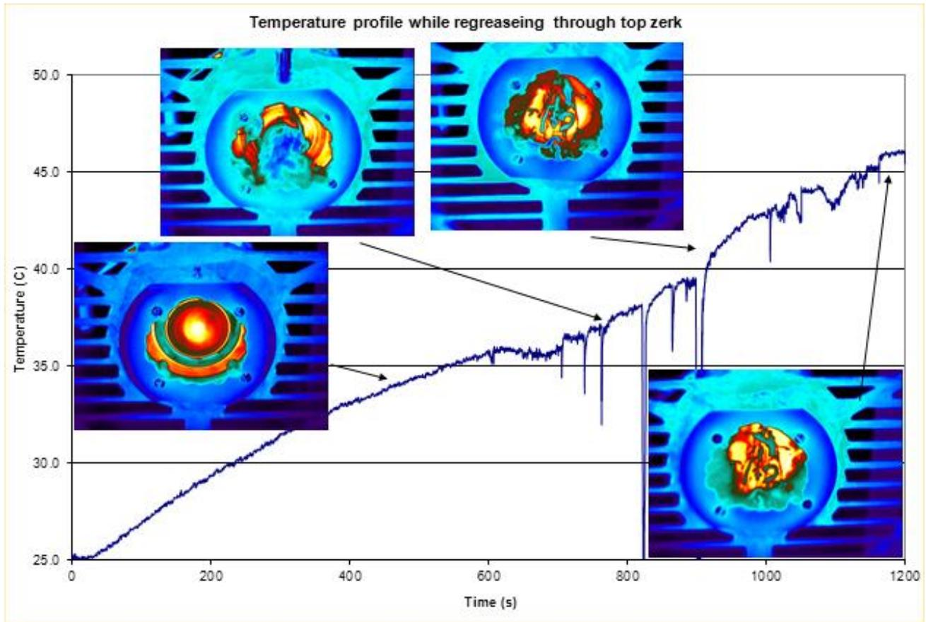
Figure 2: Increasing temperature profile on top addition of grease
