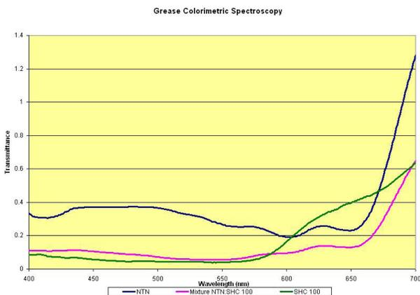
Figure 15: Colorimetric comparison of two greases, and a suspected mixture
