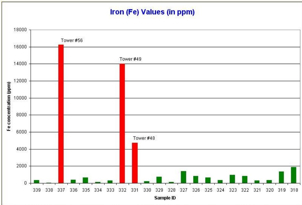
Figure 20: Graph of ferrous debris levels in multiple wind turbine main bearings, indicating abnormally high wear levels in three of the turbines in this farm.
