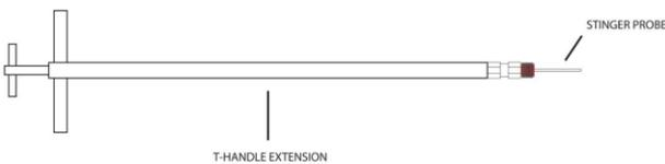
Figure 7: Grease sampler in t-handle extension
