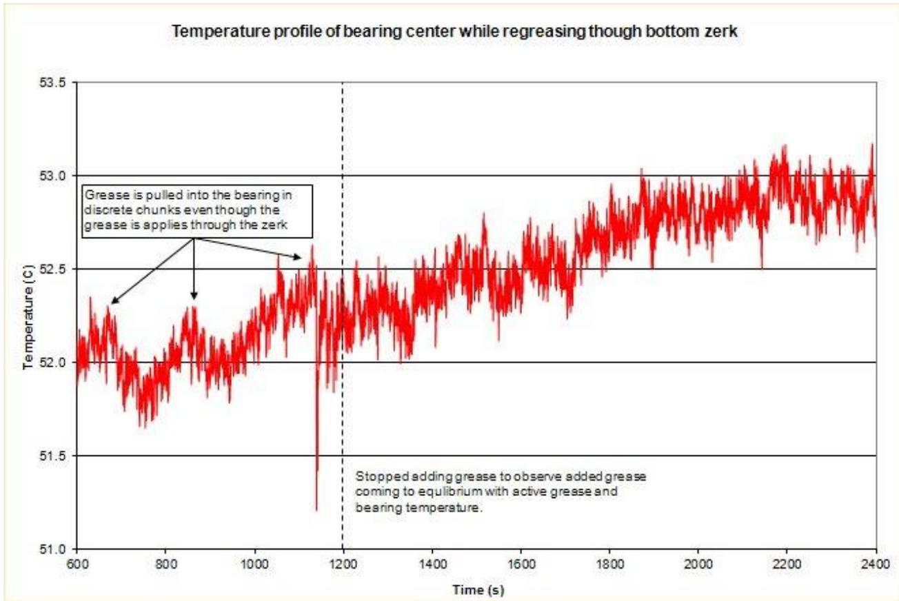
Figure 3: Increasing temperature profile on bottom addition of grease
