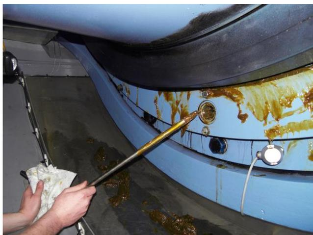
Figure 19: The full Grease Thief is removed from the drain of a 2MW wind turbine, and can be submitted for streamlined routine analysis for grease and bearing condition assessment. (Oelcheck Labs, Germany)
