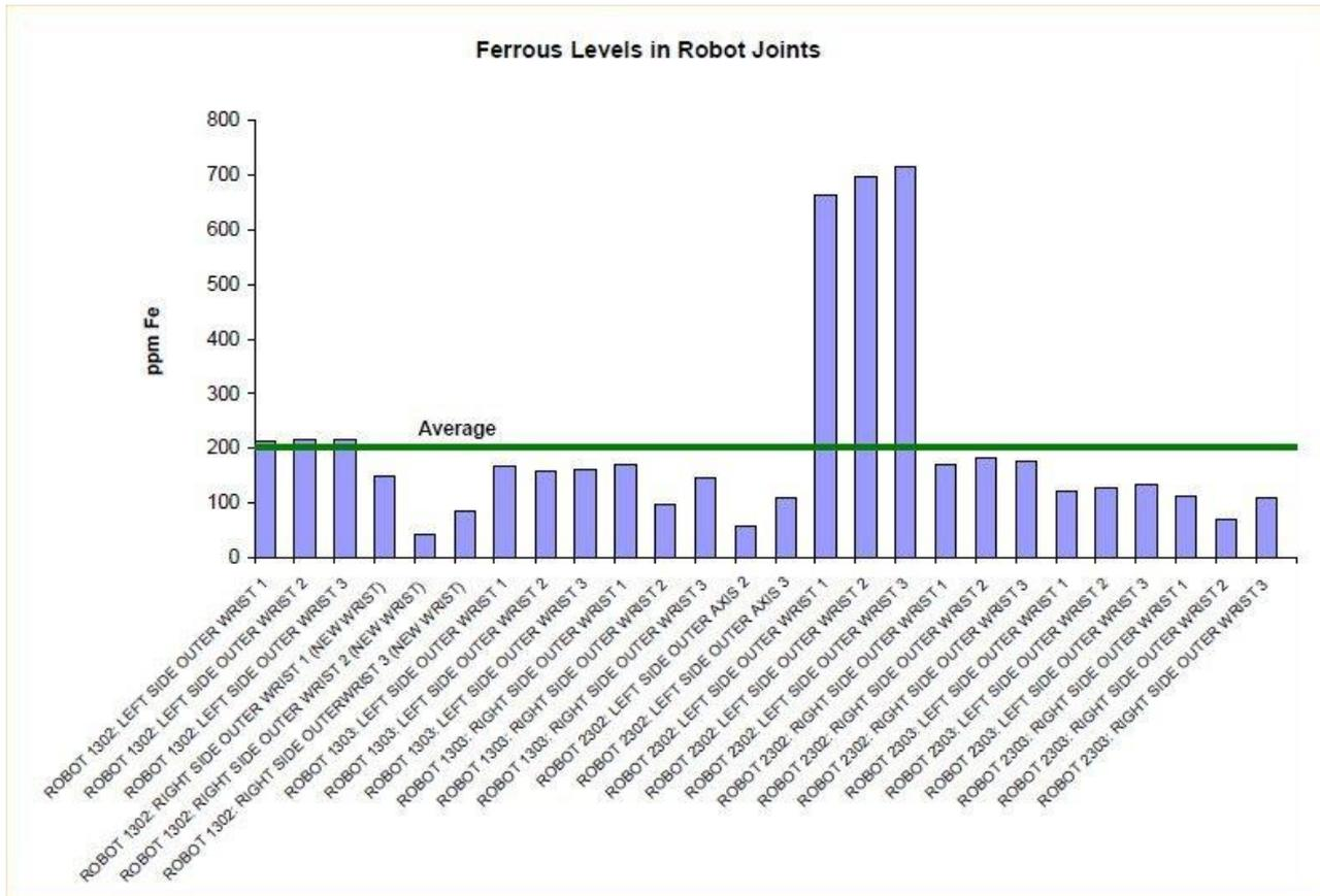
Figure 21: Graph of multiple robot drive joints, indicating abnormally high wear levels in one robot.
