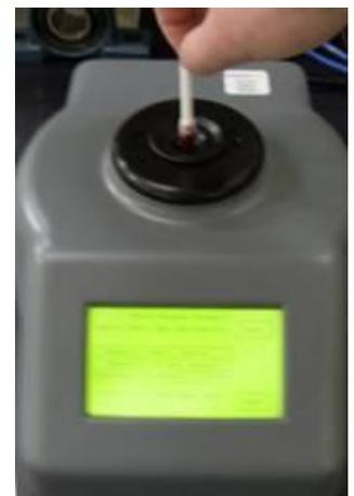
Figure 11: Hall-effect (FdM+) sensor and Grease
