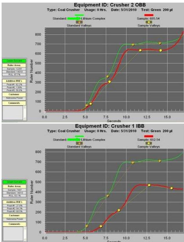
Figure 13: RULER test to evaluate two greases from similar operating equipment, with the lower showing more rapid loss of anti-oxidant
