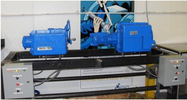
Figure 8: Motor Operated Valve (gearbox) test stand
