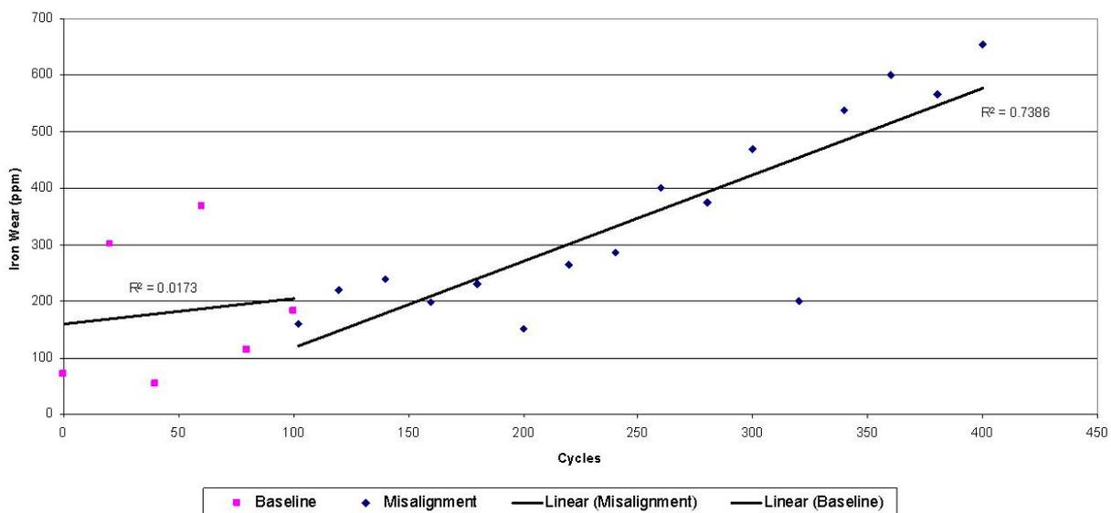
Figure 12: Increase in wear rate on pinion misalignment
