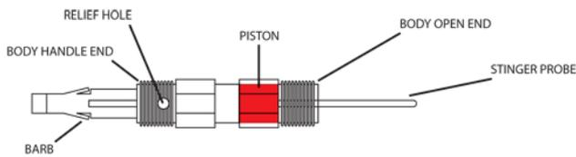
Figure 6: Grease sampler for gearbox testing
