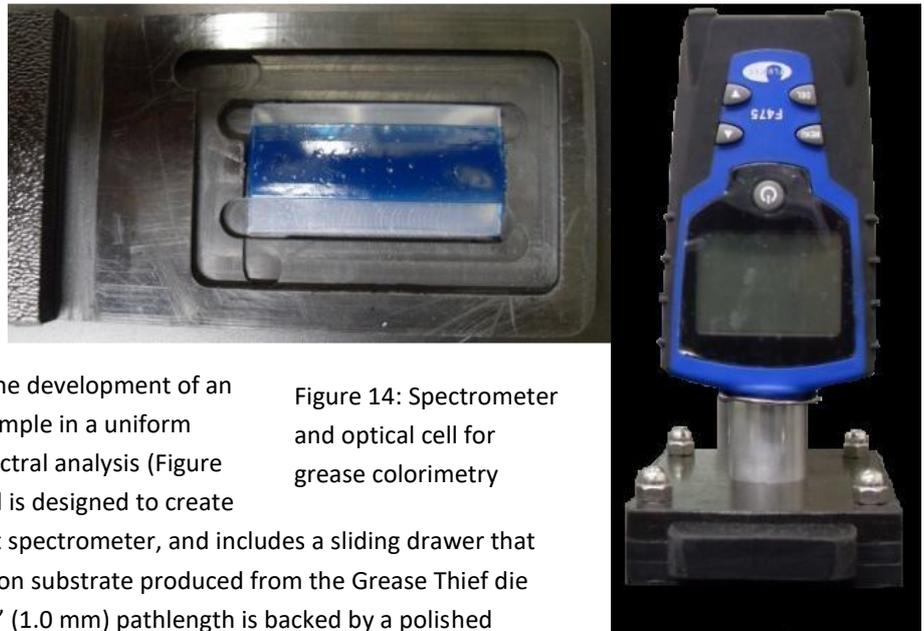
Figure 14: Spectrometer and optical cell for grease colorimetry
